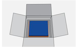
The Payload box (D) can be found below the refrigerants. The Payload box (D) holds the product Carton
