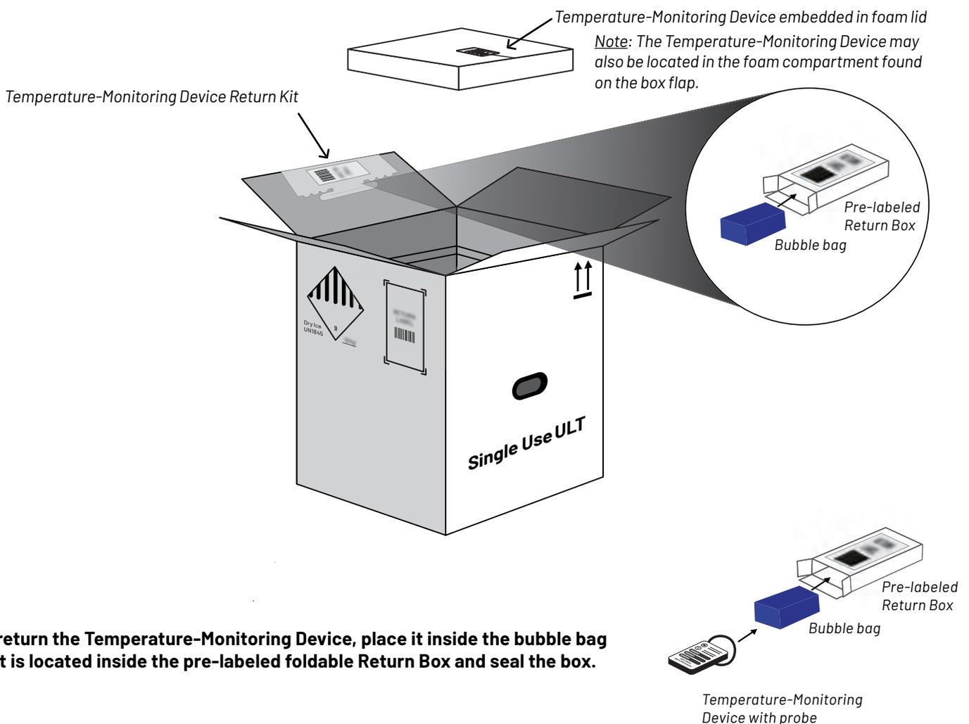
**To return the Temperature-Monitoring Device, place it inside the bubble bag that is located inside the pre-labeled foldable Return Box and seal the box.**
